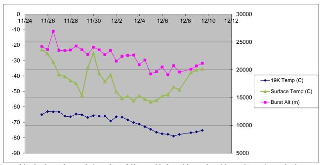
Burst altitudes have dropped abruptly to 20km and below this week, with no change in method or equipment (inflated balloons are still given 15-25 mins to equilibrate in SOB). Burst altitude does not seem as responsive to surface temp at launch, but perhaps more closely correlated to temperature at altitude, which dropped in the last week?
