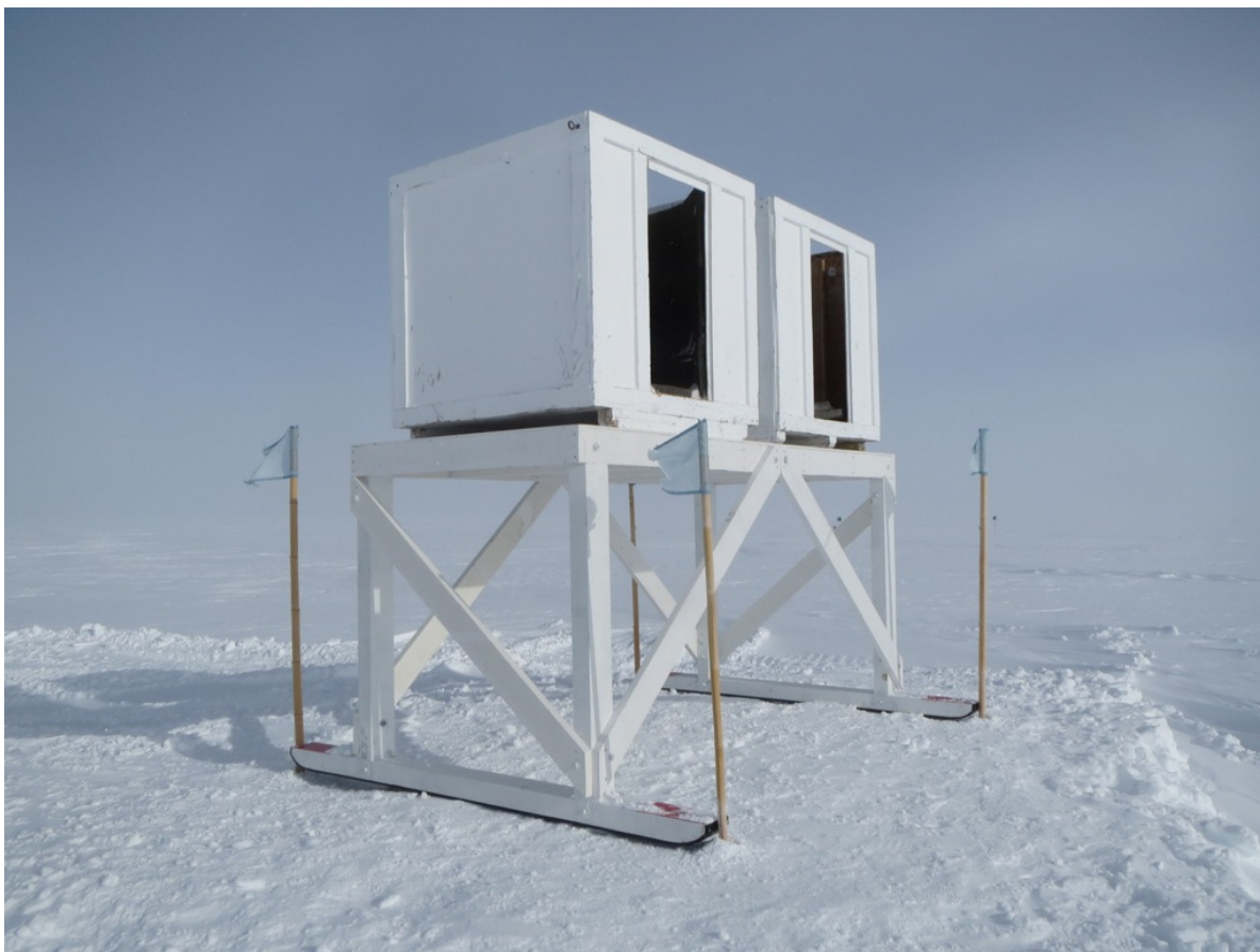
5/19: The SODAR on its new frame – with very slippery skis!
