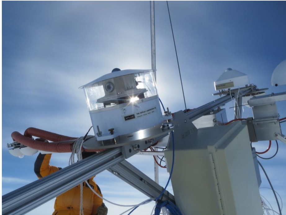
A halo around the NOAA downwelling pyranometer during Koni Steffan's solar instrument raise. -HJ.
