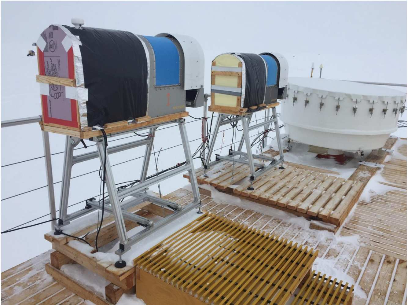
The MWRs sit ready for the winter under new insulated blankets. SWD
