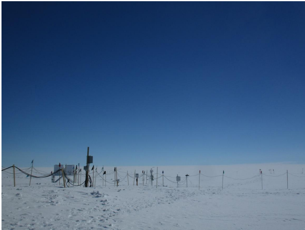
Cables and footpaths radiate from the precipitation suite. SWD
