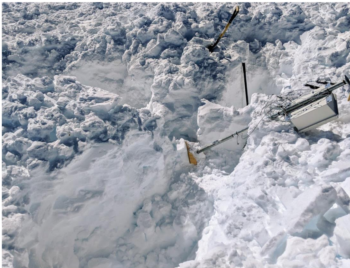
Three large holes dug to remove the Hotplate stand and anchors. (Photo: Marci Beitch, 2018-06-20)
