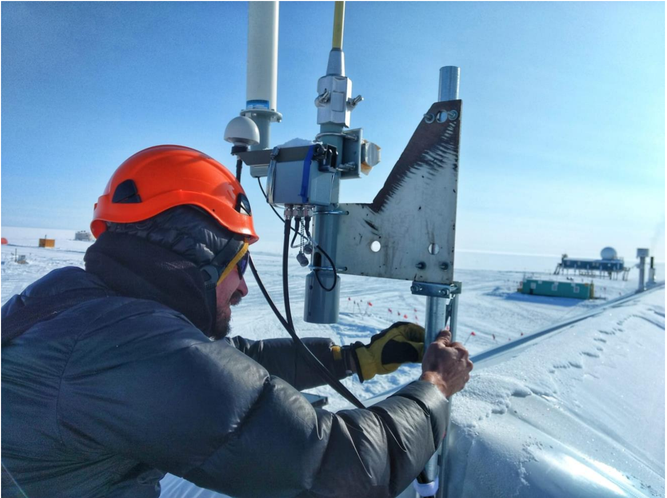
Nate Bowker making final adjustments to the radiosonde antenna on the SMG, 2019-08-23
