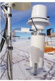
We spent a couple of afternoons working on the tower this week as we replaced the fluxtower aspirated shields with the Summit Station 'upgraded' versions. The new shields (lower right) have a longer, wider inlet, and a base plate to mitigate heating from solar reflection. It is hoped the new shields will not get 'plugged' with ice like the original versions (upper right).
