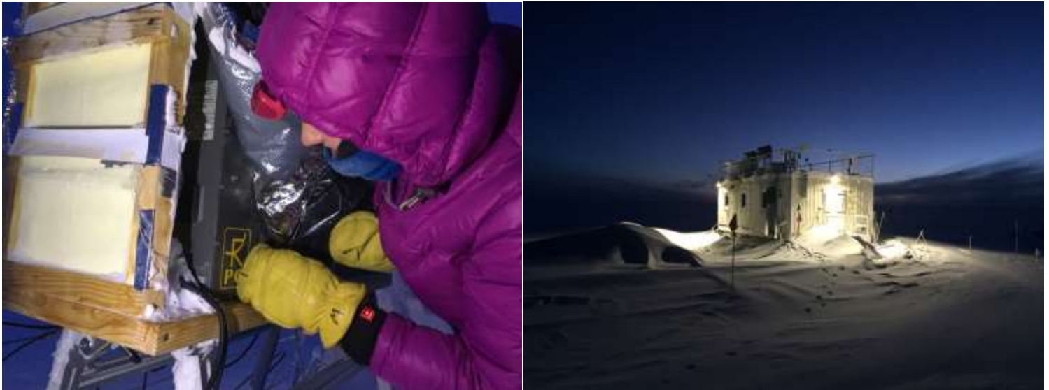
Left: 2019-12-05: ICECAPS Tech Jess investigating the HATPRO Microwave Radiometer (MWR) connectivity issues.
