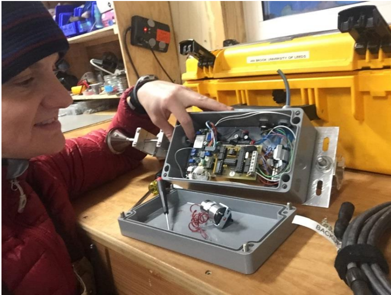
Left: 2019-12-10: ICECAPS Tech Jess replacing the pump in the CLASP.
