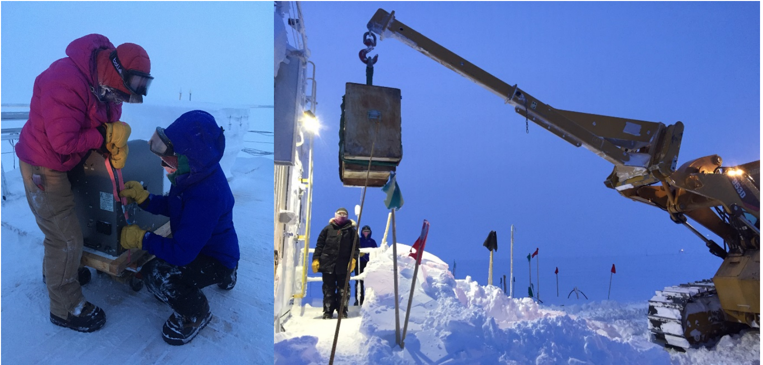
Left: 2020-01-20 1330Z: Summit Science Techs Jess and Holly secure the HATPRO MWR to its crate base. Right: 2020-01-20 1400Z: The 953 with stinger attachment lowering HATPRO MWR onto MSF front deck.
