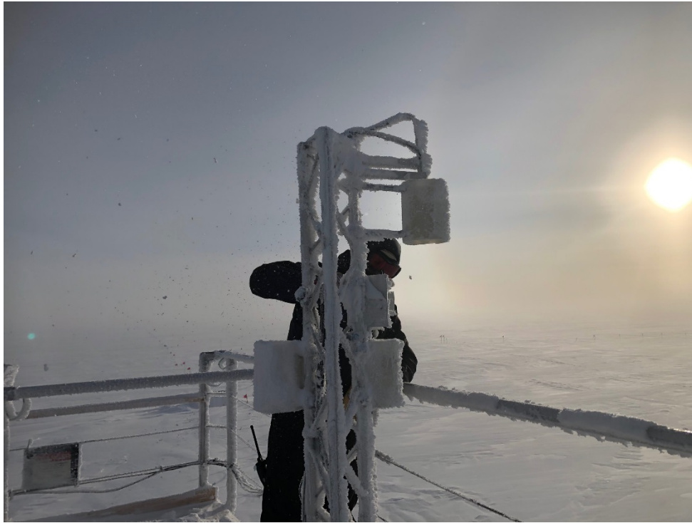
Nate removing frost from ACE instruments on a somewhat windy day. Photo Kathy Schrader
