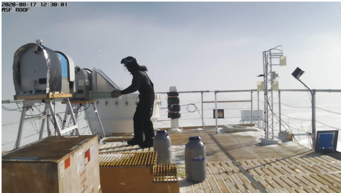
Performing liquid nitrogen calibrations for the HATPRO.
