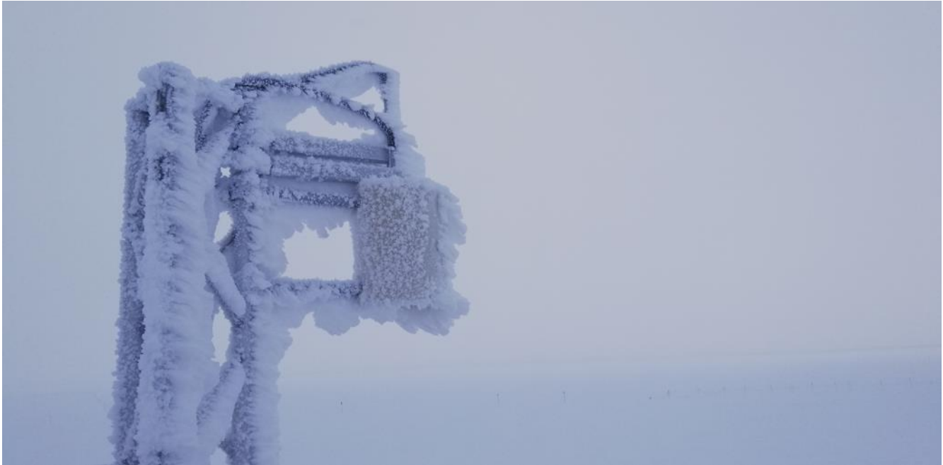
Heavy frost build up on the SKYOPC inlet during a thick freezing fog event on 2020-10-09.
