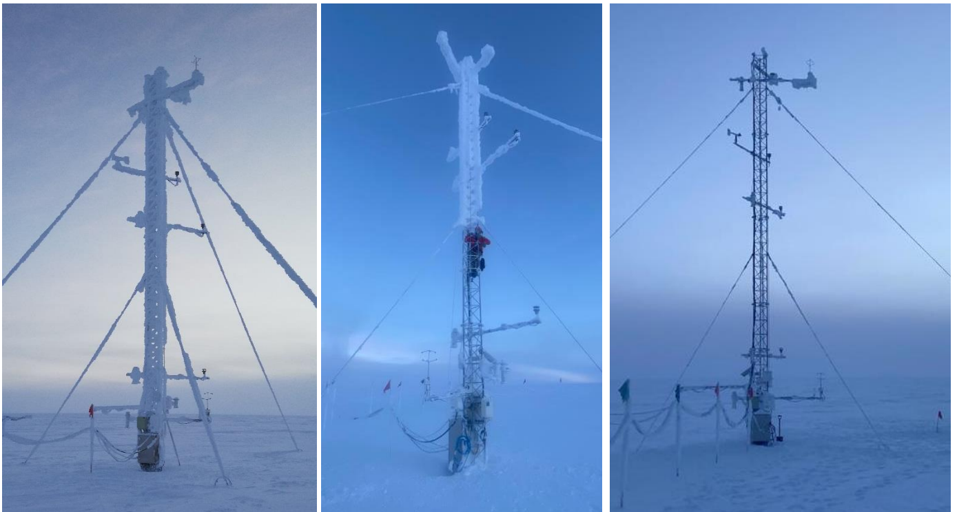
TAWO Met tower, before, during and after cleaning on 2021-01-31
