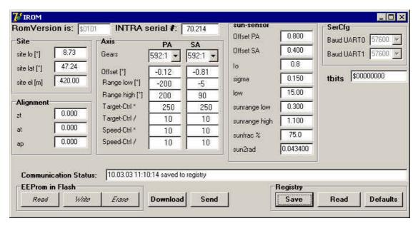
Some of these parameters are informative only, but most of them are actually used in computations by the firmware. Some of the parameters are defined at the factory (M), some are defined by the user (U) and some are computed/updated (P) by the firmware during operation.
