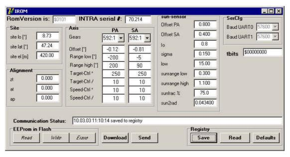
Now please enter the parameters of your site in the 3 fields inside the Site-frame. Longitude (East is positive<sup>2</sup>), latitude (north is positive) and elevation (m above sea level). Then click Send followed by a click to the Write button in the "EEProm in Flash"-frame. The new settings are now in the RAM of the controller and also in its ROM (emulated in flash). Hence during subsequent the power ups, INTRA will come up with these settings read from ROM during power up.
