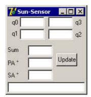
When clicking the Update button, the q0 to q3 fields display the signals of the 4 quadrant sensor. The Sum displays the sum of q0..q3, and PA, SA the pointing error as computed from q0..q3. The field at the low rim is used to display communication status messages.
