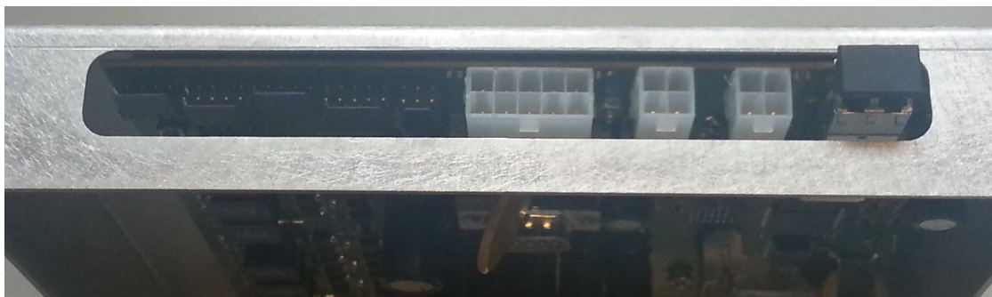
Figure 1.1 The sockets of the Intra Controller Board Version 2 (icb-2). From left to right: Encoder PA, Motor PA, Encoder SA, Motor SA, Sun-sensor, X1 Main socket, Heater PA, Heater SA, LAN-socket (not used)
