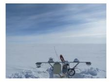
Assemble the tripod on the ground near the instruments. When ready to lift, have one person at each leg and a fourth person directing traffic. Slowly walk the legs in towards the center, bracing the large rectangular plates against your body securely. The person directing traffic will ensure that the top is centered directly over the instruments so there will be no pendulum effect when the raise happens.
