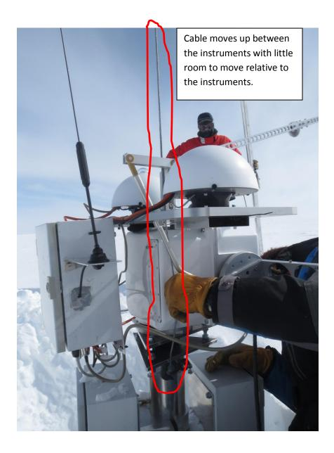
5. Tie a tagline below the instruments to ensure a smooth, controlled raise and lower. Again, ensure that no cables or cords will be pinched with these knots. \*\*\* VERY IMPORTANT: See step 9 for the non-tracking stand\*\*\*
