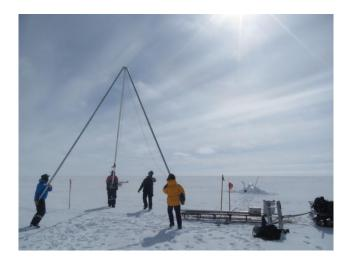
Koni Steffen and his group will raise the two solar suites that are halfway between TAWO and the MSF when neededusually every few years. They bring their own collapsible tripod setup with a crank to raise the instruments out of the snow before putting extensions on the stands. The following steps document how to safely raise and lower the instruments via installation of extension stands.
