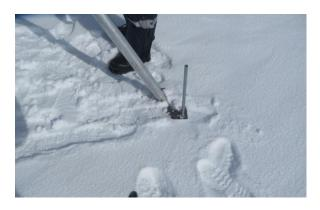
3. Crank the cable and hook down to the person handling the solar stand.
